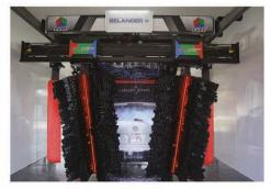
The Smart Wheels tilt inward at the top to cover the upper portions of vehicles, and inward at the bottom to clean the lower sides on the second pass. Match that with angled passes at the backside for difficult SUV contours, and you have a precision wash. In other words, the Cube knows the shape of the vehicle and maintains optimal positioning and cleaning angles.
